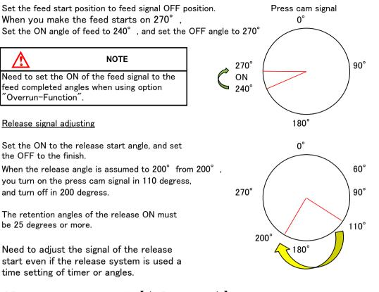
◆Release setting in the controller【(\_\_Release Mode)】
