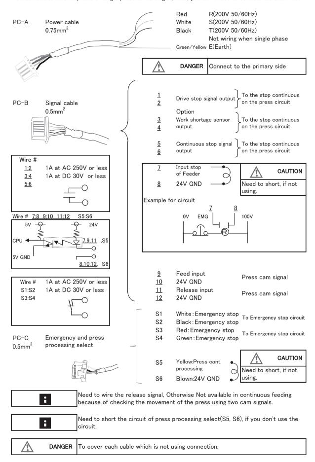
The receptacles of PC-A, PC-B, PC-C are placed inside the connecting cover.
